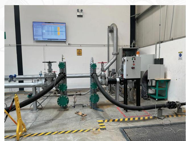
he Pump Test Bench provides advanced technology to monitor and control the process of testing the pumps
