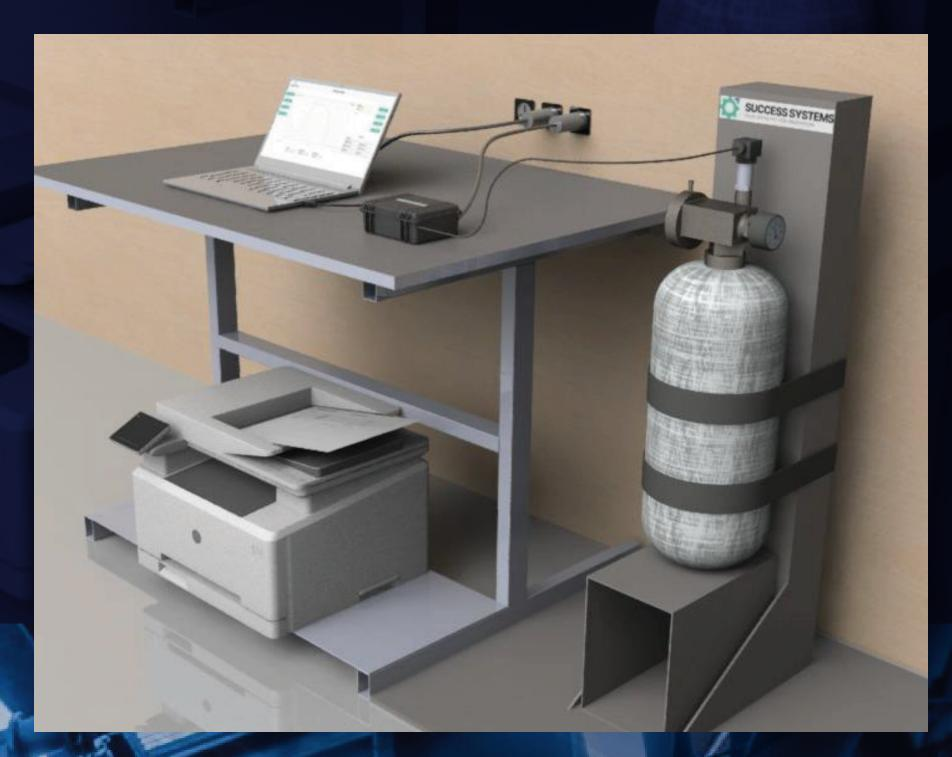
The system is capable of testing nearly any pressure level. Typically, we supply it with a range of 0-1000 PSI, but this range can be extended according to the sensor's capabilities.
